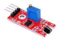
The KY-036 Metal Touch Sensor Module features a KRS13 darlington NPN transistor, the signal of which is controlled by a circuit part of which integrated type LM393 inside which there are two comparators. When you touch the bare wire bent over the transistor, which is represented by the base of the transistor, the 50 Hz signal around us in a modern home or office is injected into a high gain amplifier.
