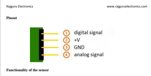
The sensor has 3 main components on its circuit board. First, the sensor unit at the front of the module which measures the area physically and sends an analog signal to the second unit, the amplifier. The amplifier amplifies the signal, according to the resistant value of the potentiometer, and sends the signal to the analog output of the module.
